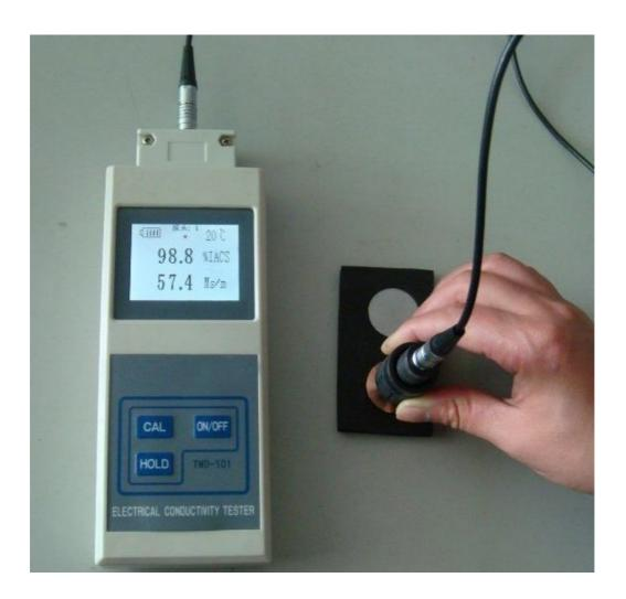
TMD-101 is a kind of eddy current electrical conductivity meter, which is designed for q uick & convenient measurement of material property, such as material separate, quality co ntrol, material state check and so on. It uses the electromagnetism testing principle. Testin g objects focus on non-ferromagnetic material.
